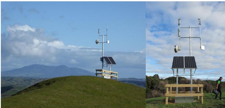
*The light wire towers stand approximately 7 m tall with antennae attached, and are solar powered.*
